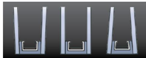
This illustration shows how the BarrierXP ThermD Spacer expands and contracts with the window glass. In warmer weather, the spacer allows for expansion. In colder weather, the spacer contracts with the glass. The spacer's flexibility ensures that the sealant used is not compromised and won't separate from the metal or the glass. This further contributes to better retention of the insulating gas.
